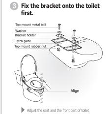
Adjust the seat and the front part of toilet back and forth so that they can correspond with before fastening the nuts.
